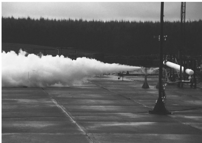
Fig. 2. LNG jet dispersion—horizontal release through a 10 mm nozzle shown.
